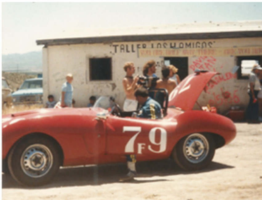
A refueling stop in an open road race between Ensenada and San Felipe, Mexico in March, 1988. An interesting thing happened in that race. At about 110 mph the hood (or bonnet) which is hinged in the front, popped up due to negative pressure over the top. The car immediately increased speed to 120 mph. due to a decrease in drag.
